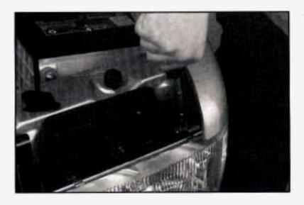
Remove the screw located behind the corner reflector in order to remove the entire corner reflector.
